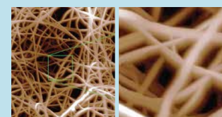
Microscope image of Nanofibres
